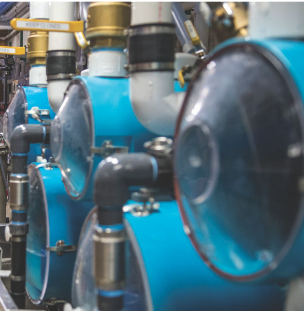
Workers at the sugaring facility in Cambridge, Vt., operate a reverse osmosis machine that removes much of the water in sap before it is boiled, saving time and reducing energy costs.
